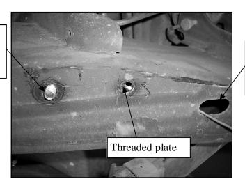
Insert threaded plate through slot in frame rail.
