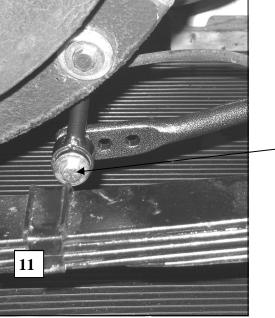
Attach end link to outer hole as shown before driving. DO NOT use inner holes until first driving vehicle with end link in outer position.
